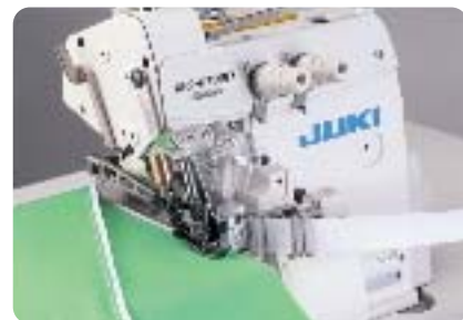
● Rolling in tape MO-6745D-FF4-360/N077 (N077: Clean finish top and bottom)
