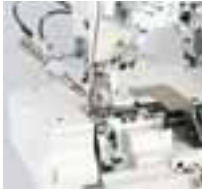
Pneumatic type needle thread / looper thread trimming device
