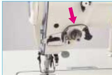
Bobbin thread is retained with a low tension, thereby preventing stitching troubles at the start of sewing
