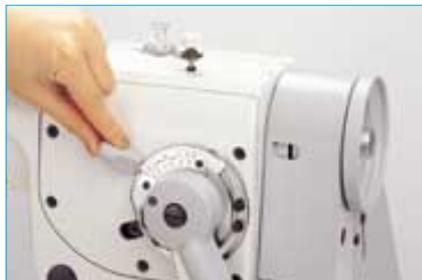
The machine is equipped, as standard, with a needle throw direction change-over mechanism
