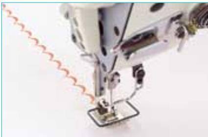
The position of needle entry is easily determined
