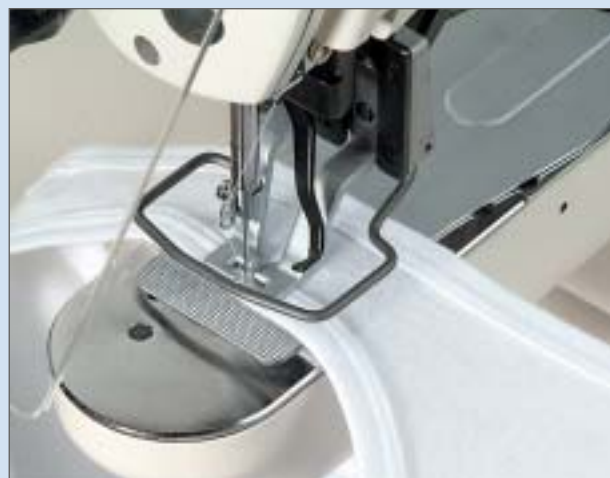
❖ M type (Bartacking shoulder of running shirt)
