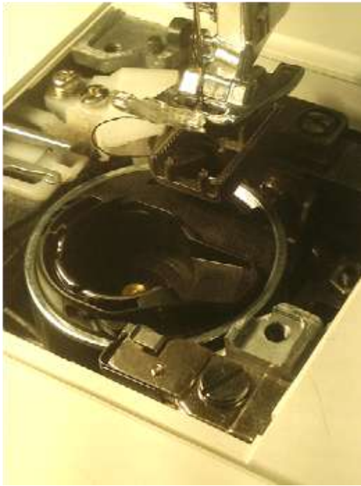
Top left remove 2 holding screws
