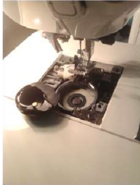
Top right remove plate, have needle at its highest point
