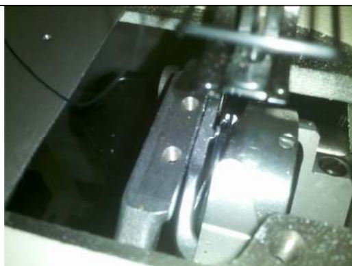
Feeder removed note finger located in bobbin basket
