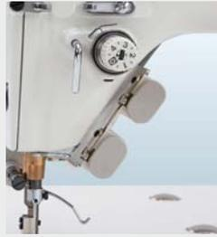
★With the option switch, the operator can select one of various optional features, which include the needle up/down compensation, 1-stitch compensation, reverse-stitch compensation, auto-lifter, thread trimming, and cancellation of automatic reverse stitching at the ending of sewing.
