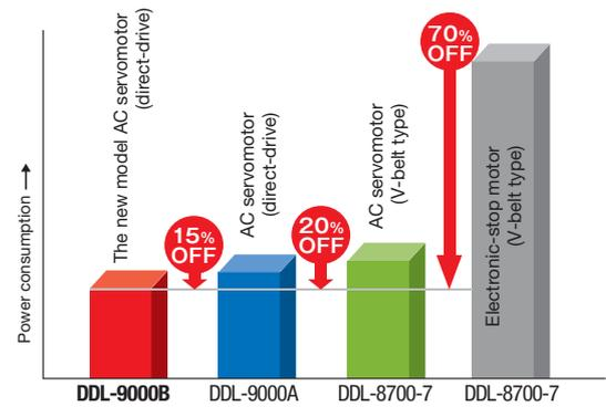
\*When the DDL-9000B runs under the energy-saving mode, the sewing machine availability factor is 25%
