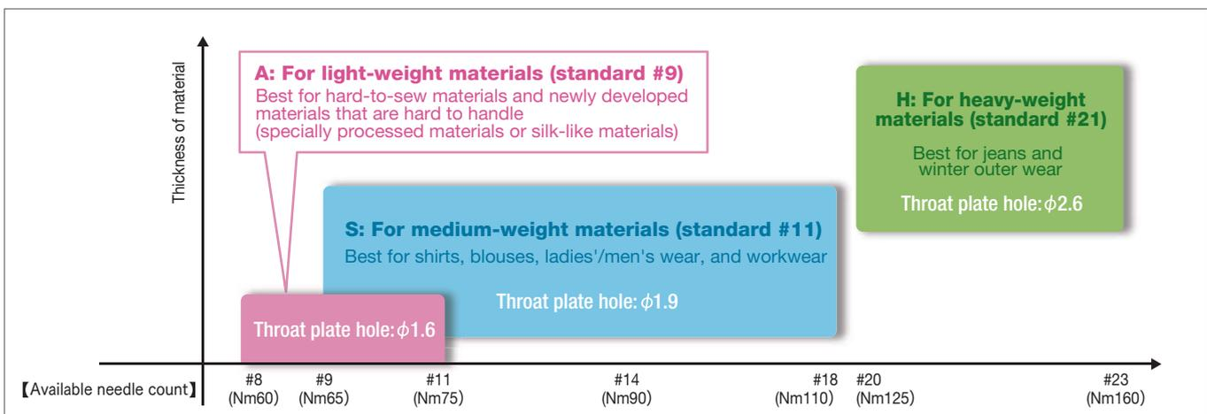
【 The sewing range in which the machine can sew with the factory-attached standard gauge 】
