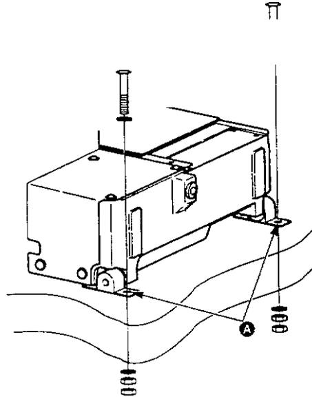
(3) Lift the sewing machine head, fit the holes of hinges **B** to the holes of table and fix as shown in the figure.
