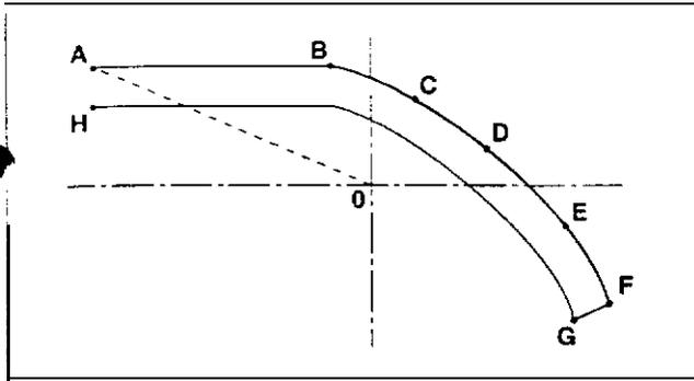
When inputting A-S-C-D-E-F using the function of the double-stitch sewing, double-stitch sewing of A-B-C-C-E-F-G-H can be made.
