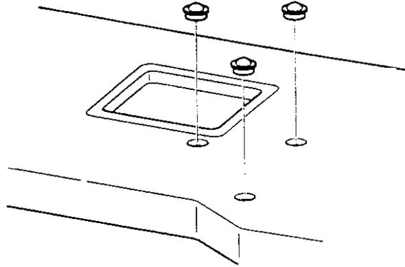
(2) Fit the holes of hinges **A** to the holes of table and fix as shown in the figure,
