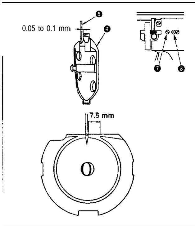
4) Loosen shuttle race screw ⑦ , and adjust the longitudinal position of the shuttle race. To do this adjustment, turn shuttle race adjusting shaft ⑧ clockwise or counterclockwise to provide a 0.05 to 0.1 mm clearance between needle ⑤ and and the blade point of shuttle ④ .
