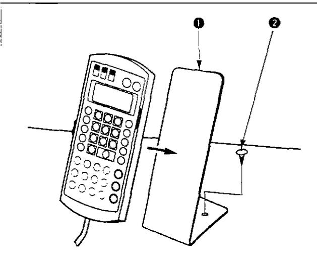
Fix operation box attaching plate O on the table with wood screw ②.
