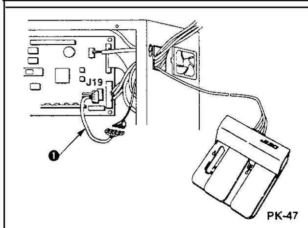
In case PK-47 (GPK47001 OAO) is used for the foot switch, use pedal switch shifting cable (M90255800A0) 0.
