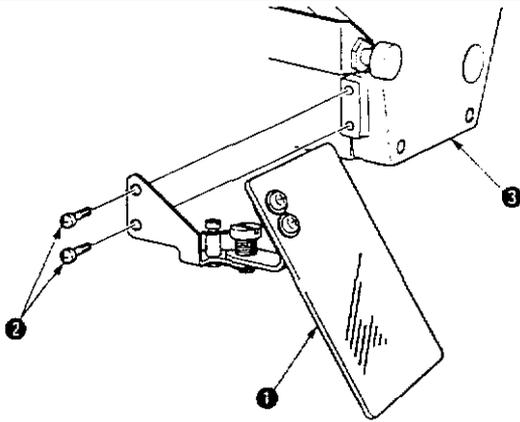
Use eye protection cover 0 after securely attaching it on face plate cover 3 with screw 2.
