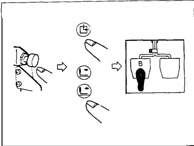
1) As "Stop-key is pressed" is shown on the operation panel, press again the temporary stop switch and actuate the thread trimmer.
