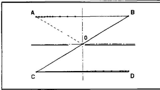
At the start, make the linear sewing, **A-B-C-D**, and sewing pitch of 2.5 mm. And, the condensation stitching which makes the sewing pitch finer, is to be performed at the **start** and end of sewing.
