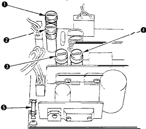
The machine uses the following five fuses :
