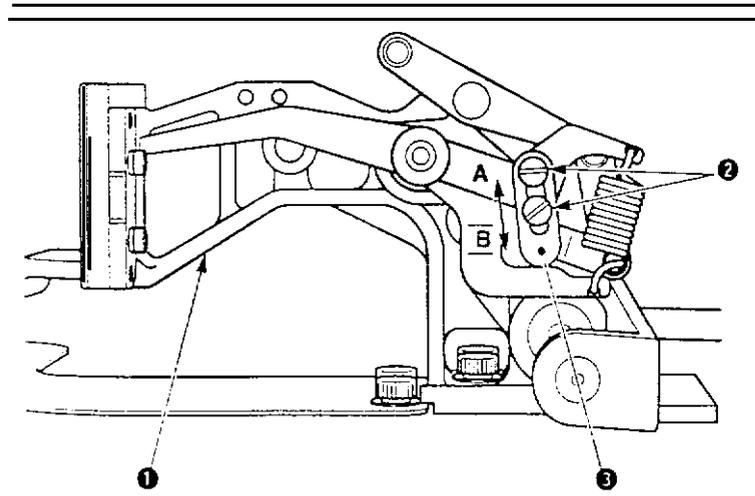
1) Loosen screws ② located on the right and left sides of feed bracket ① . Moving cloth presser stopper ③ to the direction B will increase the height of feeding frame.
