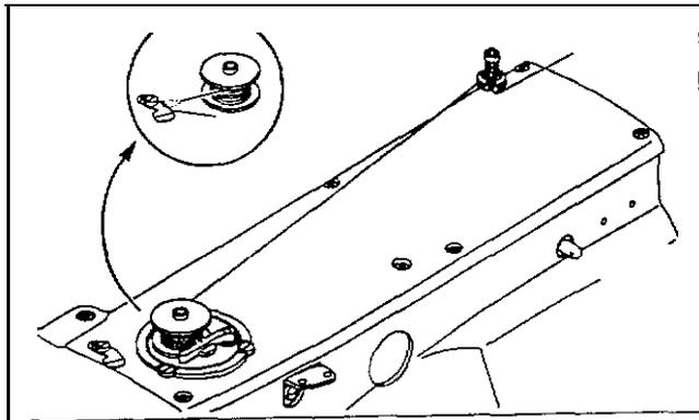
Thread the bobbin winder and wind the thread onto the bobbin as illustrated in the figure.
