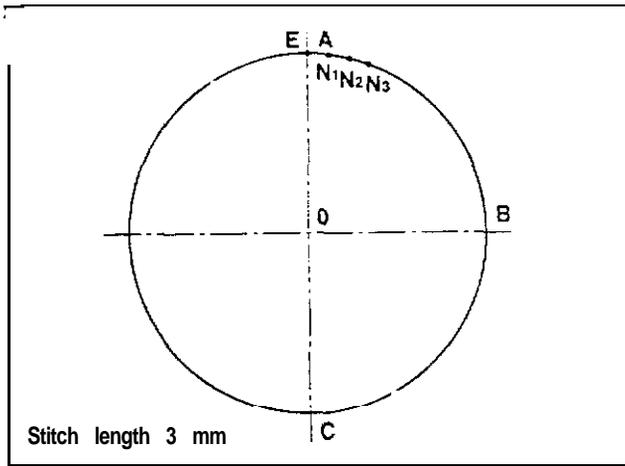
After the circle, ABCE, is made. from the end point of the circle, E, the stitches are made so as to overlap N<sub>1</sub>, N<sub>2</sub> and N<sub>3</sub>.
