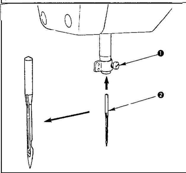
Loosen setscrew **1** and hold needle @with the long groove facing toward you. Then fully insert it into the hole in the needle bar. and tighten setscrew **1**.
