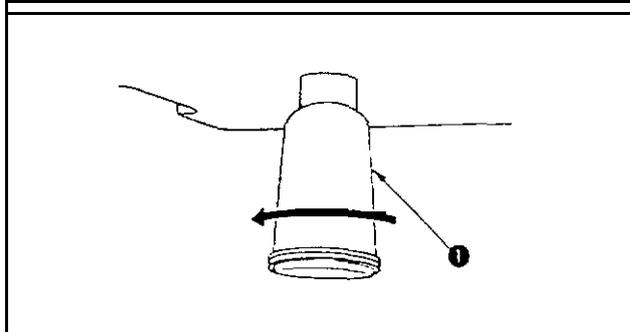
When polyethylene oiler **0** becomes filled with oil, remove it and drain the oil.
