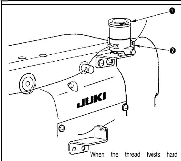
Fix silicon oil tank **1** (MAXAP30EX00) with the magnet.
