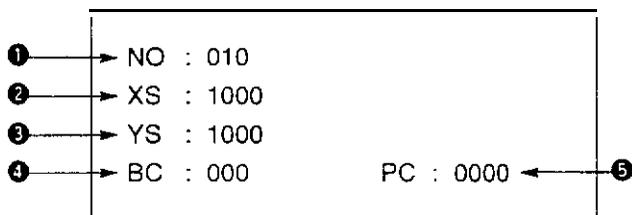
○ Indication of Pattern No. : Can be changed by No. key and Numerical key.
