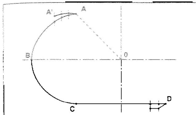
At first, input the arc ABC and the line CD. Then, input 3 stitches at the sewing start and 2 stitches at the sewing end.
