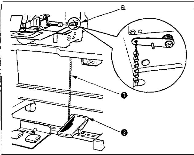
Connect the machine ① and manual pedal ② with chain ③.
