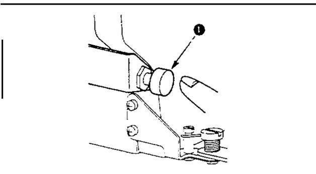
Press the temporary stop switch **0** while the sewing machine is in operation.
