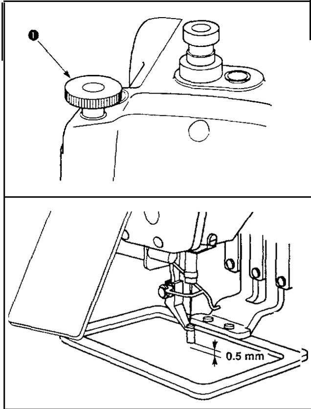
Turn handwheel, and adjust so that a clearance of 0.5 mm (thickness of the needle thread used) is provided between the bottom end of the intermediate presser and the material when the needle is brought to the lowest point of its stroke by turning the knob **0**.
