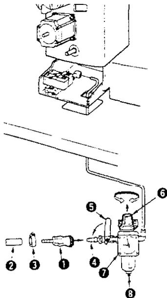
Open air cock 5, pull up the knob 6 of air regulator and turn it to adjust so that the air pressure gauge 7 indicates 0.5 to 0.55 MPa (5 to 5.5 kgf / cm<sup>2</sup>). Then press the knob to maintain the pressure value.
