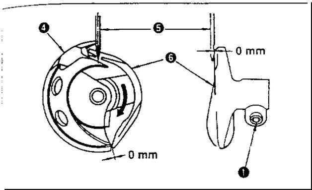
3 ) Adjust so that the point of shuttle ④ meets the center of needle ⑤ , and that a clearance of 0 mm is provided between the front end face of driver ⑥ and needle as the front end face of driver receives needle to prevent the needle from being bent. Then tighten setscrew ① .
